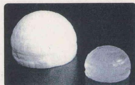
**A cast and dried mixture of silica powder and a synthetic resin, left, is transformed into a silica glass object, right, by using heat.**
