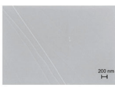
d) Homogenous Al 2 O 3 film deposition onto graphene by two-step ALD technique.
